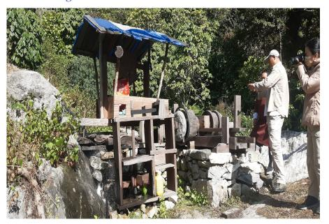
The multiple farm produce processing machine using clean energy source that is from a nearby stream is agreed to be established in Thangrong Daksa. The key innovator Tshewang, 46 of Thangrong Daksa developed a flour mill, milk churner and tegma machine using only wood, stone and a pair of bearing with some rubber tubes which is run on the energy from free flowing stream. It is a nicely arranged
